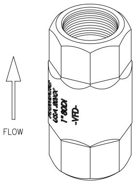
Max Temp 180°F (82°C) Max Pressure 600psi (41bar)
