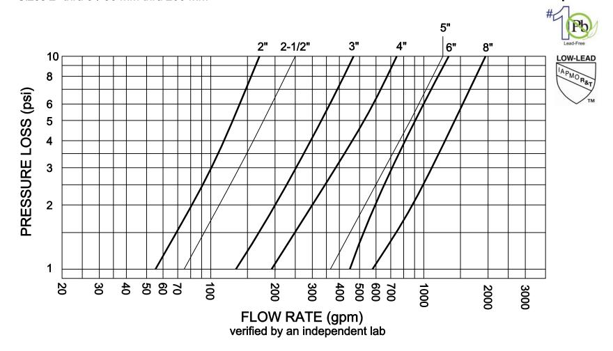
Note: For longer service life & higher efficiencies it is not recommended that flow velocities exceed 10 feet/second
